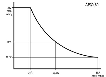
These compact autoranging bench or systems power supplies use a switch-mode topology to provide a wide range of adjustable voltage and current combinations within a 3 kilowatt power envelope.
