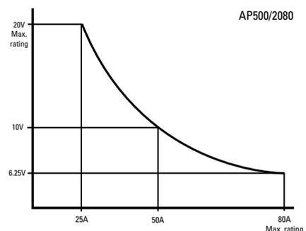
These compact autoranging bench or systems power supplies use a switch-mode topology to provide a wide range of adjustable voltage and current combinations within a 1 kilowatt power envelope.
